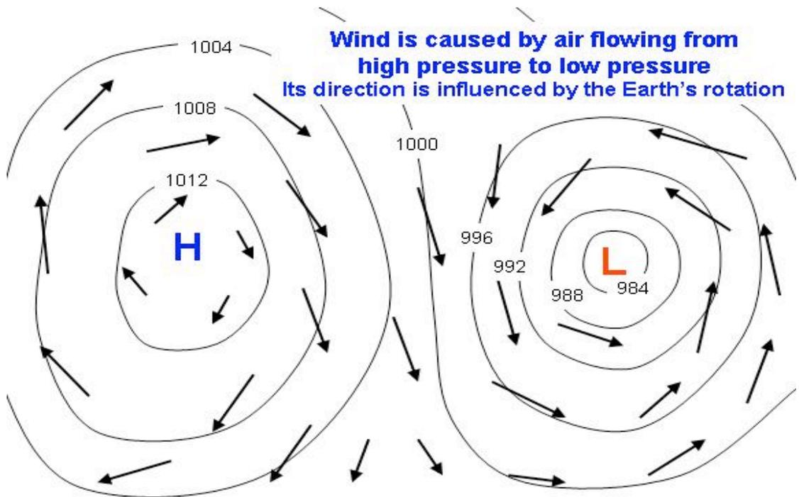
Forces acting on Wind: 1) Pressure Gradient, 2) Friction, 3) Coriolis, 4) Centrifugal
